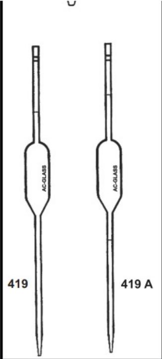
**PIPETA VOLUMÉTRICA, CALIBRADA A 20°C, "CLASSE A", COM UM OU DOIS TRAÇOS . AC-GLASS**
